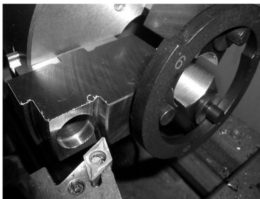
Turning the jaws (internal clamping)
