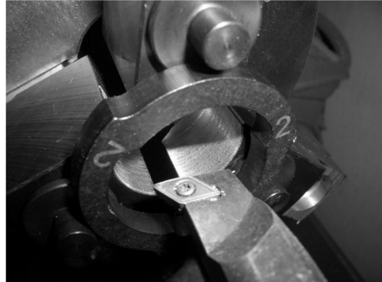
Turning the jaws (external clamping)
